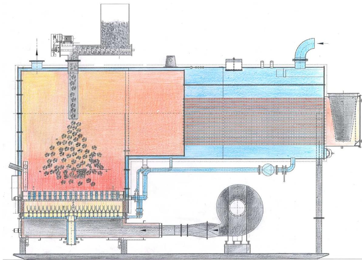
Next to running your boiler fully automatic, it is also very important to burn solid fuels as environmentally friendly as possible. This method, which combines both is also the fluidized bed combustion. In this combustion fuel parts are kept "floating" in hot combustion air and sand with a combustion temperature that does not exceed 900°C. One can accomplish the following:
